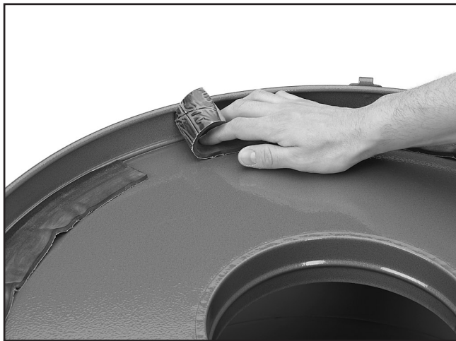
Figure 34. Applying dust collection drum lid gasket.
